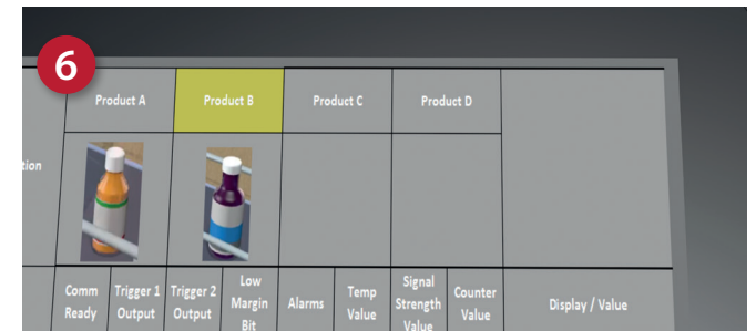
6. Smart sensors have new parameters set for Product B – machine ready to start
